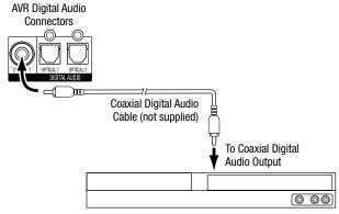
Coaxial-Equipped Source Device
