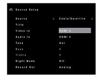
Select "Audio In" and use the left/right arrow buttons to select the audio input connector you want to assign to the Source button.
