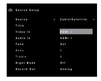
Select "Video In" and use the left/right arrow buttons to select the video input connector you want to assign to the Source Selector button. Press the OK button.
