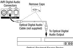
Optical-Equipped Source Device
