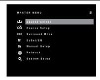
The Master menu consists of seven submenus: Source Select, Source Setup, Surround Mode, EzSet/EQ, Manual Setup, Network and System Setup.
