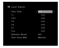
All of the system's speakers will appear with their current level settings. You can adjust each speaker's level between  $-10 \, \text{dB}$  and  $+10 \, \text{dB}$  in  $1 \, \text{dB}$  increments.
