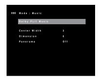
**Center Width:** This setting affects how vocals sound through the three front speakers. A lower number focuses the vocal information tightly on the center channel. Higher numbers (up to 7) broaden the vocal soundstage. Use the Left/Right buttons to adjust this setting.
